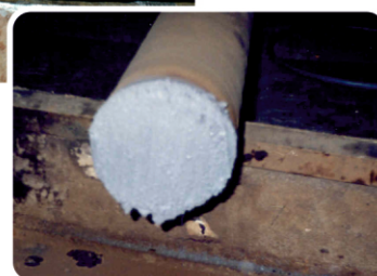
An example of cutting rolled metal 150mm thick of steel 12x18H10T
