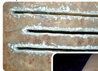
An example of cutting a rough part of SCh-20 60mm thick
