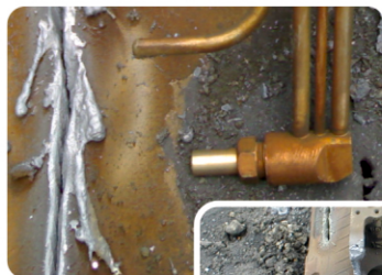
An example of cutting a sheet of metal 12x18H10T 20mm thick
