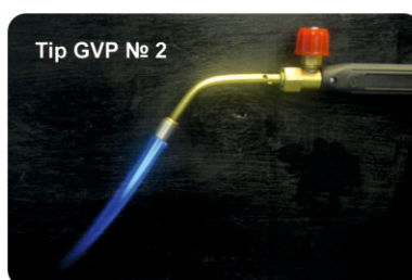
Flame core diameter – 5,5 mm Flame core length – 55 mm
