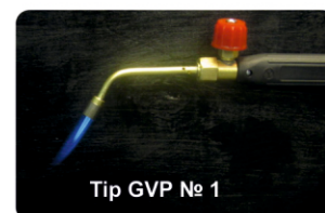
Flame core diameter – 4 mm Flame core length – 22 mm
